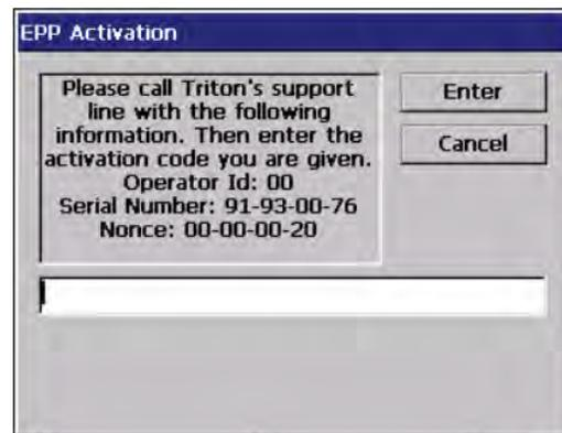
6. Enter the activation code. Press Enter on the keypad. If the code was entered correctly, the “EPP activation successful” box will appear. If the code was entered incorrectly, the “EPP activation failed” box will appear. If failed, repeat steps 4 - 6 (acquire a new code from Triton Technical Support).
