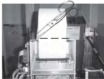
Figure 6-1. Cut paper roll here to remove.
