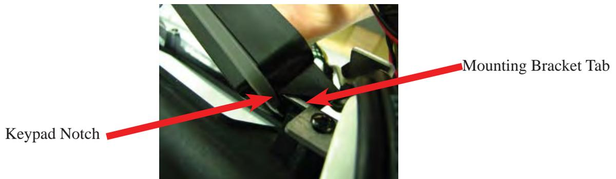
Install the top of the keypad from left to right (from the rear) ensuring the keypad gasket is sitting flush against the control panel. Using slight pressure if needed, ensure the bottom half of the keypad is also sitting flush with the control panel. Secure the keypad with the 6 screws.
