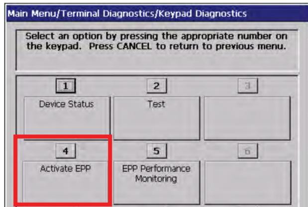
5. The following screen will appear. An activation code is required from Triton Technical Support to reactivate the T9 EPP Keypad. Contact Triton Technical Support with the “Operator Id”, “Serial Number” and “Nonce” numbers (supplied in the EPP Activation dialog box) for an activation code.
