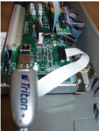
3. If your Flash drive has an indicator, it will light briefly, then extinguish. When light extinguishes, this indicates the storage device has been found by the operating system of the ATM. If your Flash drive does not have an indicator, proceed to the next step.
