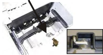
*Pull the packer back. Some cassettes allow the pusher-plate to be latched in position using the key-lock. (Insert)*
