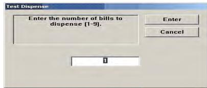
5. The Test Dispense command instructs the dispenser to dispense, *minimum*, one note from each installed and operational cassette into the reject vault. This test exercises the dispenser without sending notes to the exit.
