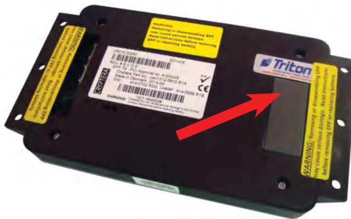
3. **DO NOT UNPLUG CURRENT BATTERY!** Obtain a replacement battery. Plug the new battery into the spare battery connection. The spare battery can be ordered at [www.atmgurus.com](http://www.atmgurus.com).
